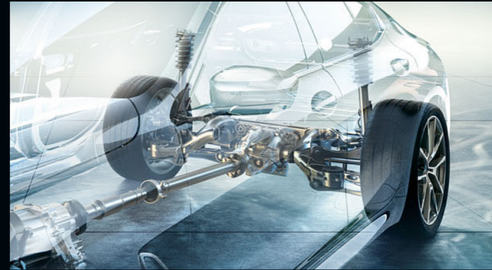
■ The M Sport differential 1,2 optimises traction and driving stability when changing lanes or accelerating out of a bend, when taking bends at high speeds or on different road surfaces. Traction is optimised with the help of an electronically operated device that reduces the difference in revolution speed between the rear wheels.
